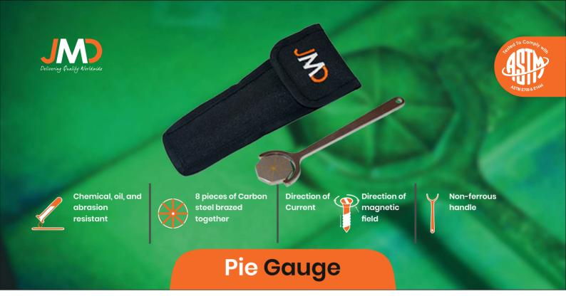
The pie gauge is a disk of highly permeable material divided into eight sections by non-ferromagnetic material. The joinings of section act as artificial defects that radiate out in different directions from the centre. The sections are furnace brazed and copper plated. The advantages of the pie gauge are that it is easy to use, and it can be used indefinitely without deterioration.
