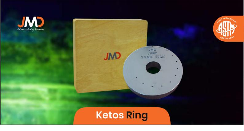
Ketos Ring is intended to be a total system check for your DC output equipment. This test gauge with subsurface discontinuities is an excellent tool that provides a quick way to confirm overall performance of your DC output machine. The Ketos Ring is meant to be a quick overall system performance indicator. The ring is to be processed by the continuous method using a 1-inch diameter central conductor.
