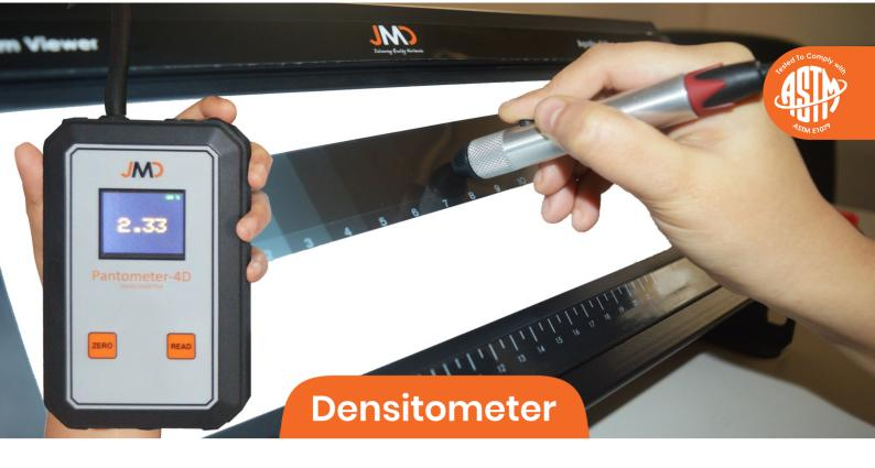
JMD Pantometer is a densitometer which is a battery-operated handheld unit used for measuring the transmitted density of X Ray film. The Pantometer has a white illumination range of 10,000cd/m² to 50,000cd/m² and has been calibrated to achieve optimum accuracy and stability for reading density. The battery can be charged with a standard USB charger which ensures an operating time of up to 10 hrs. It is manufactured as per ASTM E1079 standards.
